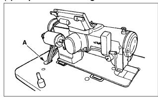
Pass the cords coming from the machine head to the underside of the table through hole A in the table.
