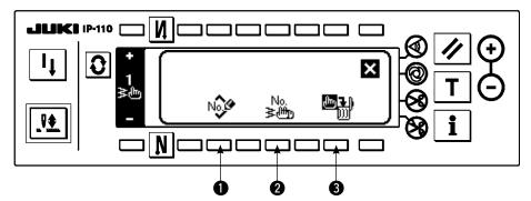
Press in the sewing shape setting screen, and the pop-up screen of registration, copy and deletion of custom pattern appears. Then registration, copy and deletion of the custom pattern can be performed.
