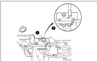
1) Remove stop plug ①, and when lightly tightening the adjustment screw ②, return the screw by approximately 0.6 turn from the stop position.
