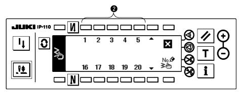
Press switch 2 corresponding to the pattern which has been registered in the custom pattern selection pop-up screen.
