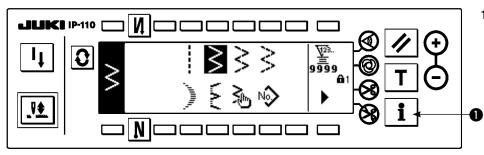
1) Press switch 1 for approximately three seconds.
