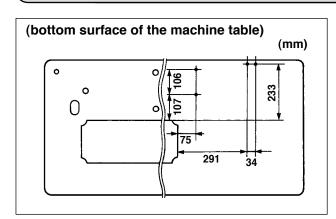
Punch dots on the positions of the setscrews of solenoid valve (asm.) and regulator (asm.) on the bottom surface of the machine table.
