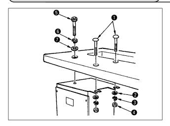
Install the electrical box on the under side of the table using round-head bolts ①, plain washers ②, spring washers ③ and nuts ④ supplied with the machine at the location illustrated, and using bolt having hexagonal indentation on the head ⑤, spring washer ⑥ and plain washer ⑦ supplied with the machine at the location illustrated.
