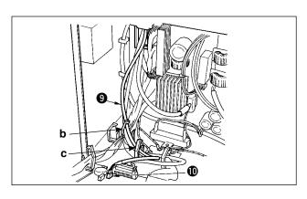
9) Insert black connector 4P white cord **9** coming from the machine head inside the electrical box through front cover through hole B, and insert it into connector CN31 **10**.
