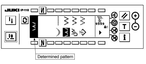
2) As an example, press the left blind stitch key and the screen on the left side appears to determine the pattern.
