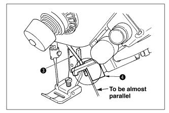
2) The top end plane of wiper 3 should be positioned to be almost parallel to the end plane of clamp head 4. Besides, set the clamp head so that the upper side is the protruding section.
