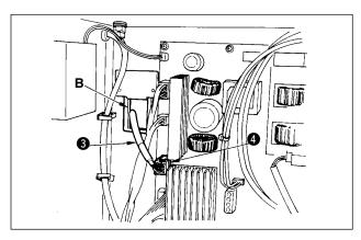
6) Insert white square connector 9P black cord 3 coming from the machine head inside the electrical box through front cover through hole B, and insert it into connector CN38 4 of the circuit board attached to the front cover.
