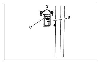
Loosen screws D and lift cord presser plate C of cord passing hole B located on the front cover to the top and temporarily tighten the plate.
