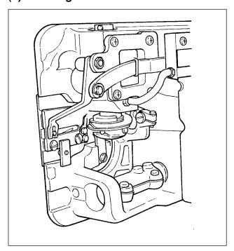
When cloth waste or the like gathers around or adheres to the hook section, trouble (defective sewing, seizure of hook, etc.) of sewing machine will be caused. Periodically clean the section.
