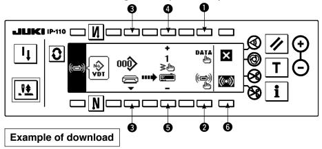
Example) Parameter file No. 70 of the media is downloaded to the condensation custom pattern at the sewing end No. 10.
