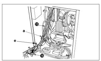
12) Insert white connector 6P three cords ( coming from the machine head inside the electrical box through front cover through hole B, pass it through cord clamps "a" and "e", and insert it into connector CN54 ( c).
