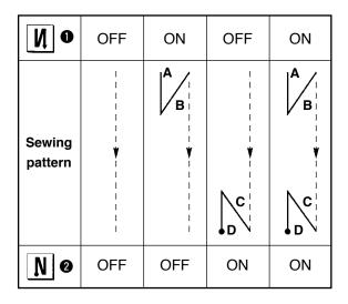
Reverse feed stitching can be set with each zigzag pattern.
