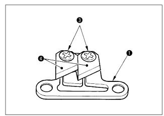
2) Remove two setscrews 3 in the knife using a precision screwdriver and remove knife (ceramic) 4 from fixing plate 1. Then replace the knife.
