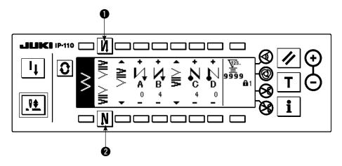
For the reverse feed stitching, there are standard condensation, 2-point condensation and condensation custom.
