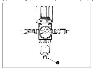
When the regulator becomes filled with water, turn knob • for drain counterclockwise.
