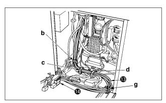
11) Insert white connector 12P cord (3) coming from the machine head inside the electrical box through front cover through hole B, pass it through cord clamps "b", "c", "d" and "g", and insert it into connector CN53 (4).
