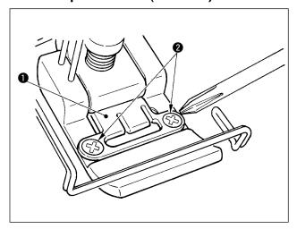
1) Remove two setscrews 2 in the knife fixing plate using a precision screwdriver and remove knife fixing plate 1.
