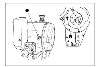
Some type of material needs to be sewn with the presser foot slightly lifted. In this case, perform this adjustment following the procedure described below.
