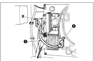
7) Insert white connector 4P black cord **5** coming from the machine head inside the electrical box through front cover through hole B, and insert it into connector CN21 **6** of the circuit board attached to the front cover.
