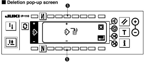
When X is pressed here, the screen returns to the former one.
