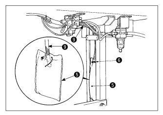
5) Insert dust bag **5** into the top end of hose **9** for dust bag and fix it with band **6** supplied with the sewing machine as accessories.
