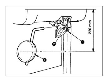
Insert knee lifter pad 1 into attaching hole 2 and tighten it with bolt 3.
