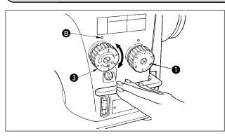
Stitch length can be reduced at the start or end of sewing. This feature is used for fastening stitch.
