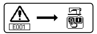
3) Remove the cause of error after turning OFF the power.
