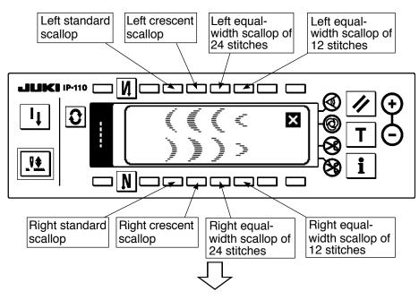
Press the switch of pattern to be selected from the screen of the left figure.
