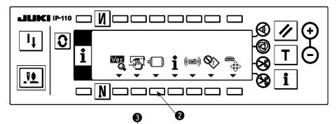
Press switch 2 for approximately three seconds.
