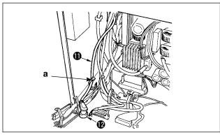
10) Insert gray round connector 7P cord **(1)** coming from the machine head inside the electrical box through front cover through hole B, pass it through cord clamp "a", and insert it into connector CN30 **(2)**.
