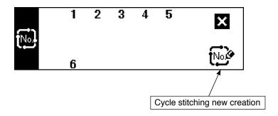
The key lock level has been set to "1" at the time of delivery, and pictographs of new creation are not displayed. When performing new creation in each mode, change the key lock level to "0". (Refer to the second screen of sewing common data setting of (1) Sewing common data of 6-15. Information.) In addition, the display of pattern No. at the time of delivery is "1" only.
