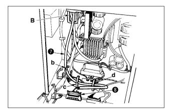
8) Insert white connector 26P cord ② coming from the control panel inside the electrical box through front cover through hole B, pass it through cord clamps "b", "c" and "d", insert it into connector CN34 ③, and lock it.
