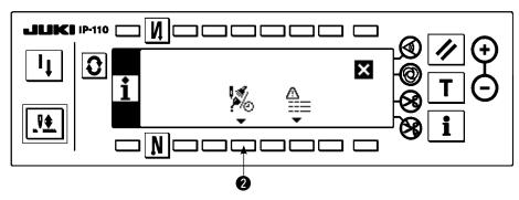
2) Press 2 to display the maintenance function screen. (For other functions, refer to the Engineer's Manual.)
