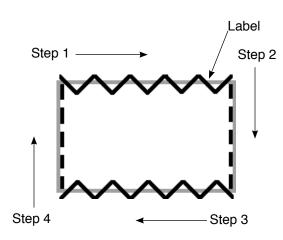
Example) In the process of label attaching, change over the zigzag patterns of constant-dimension stitching of 2-step zigzag stitch and straight stitch as shown in the figure, and perform the constant-dimension stitching.
