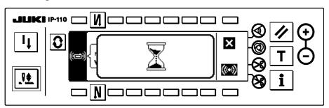
When all setting procedures have been completed, press **6** in the communication setting screen to start downloading. When the screen returns to the communication setting screen after display of the during communication screen, communication is completed.
