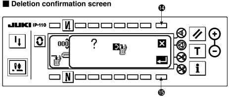
Press **(b)** and the deletion is discontinued. Then the screen returns to the file No. input screen. Press **(b)** and the deletion is executed. Then the screen returns to the file No. input screen.
