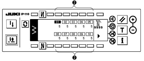
Press , in case of more than 10 steps, and programmed stitching selection screen of "11" to "20" is displayed.
