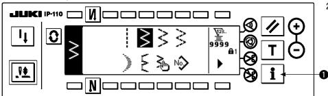
Press switch 1 for approximately three seconds.
