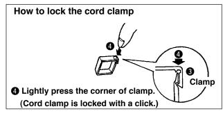
When the insertion of the connector is completed, lock the cord clamps.
