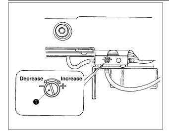
Adjustment of the amount of oil in the hook is performed with oil amount adjustment screw ①.
