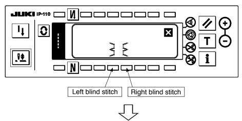
Press the switch of pattern to be selected from the screen of the left figure.
