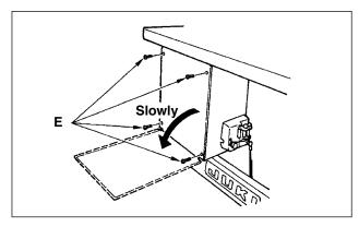
3) Remove four screws E fixing the rear cover of the electrical box. When opening the rear cover, pressing it with your hands, slowly open it by approximately 90° until it stops as illustrated.
