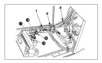
13) Insert white connector 10P cord and blue connector 2P cord coming from the machine head inside the electrical box through front cover through hole B, pass them through cord clamps "a", "e" and "f", and insert the white 10P into connector CN51 and the blue 2P into CN46 .
