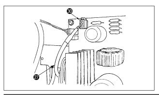
18) Insert red connector 2P side of cord 29 supplied as accessories to which red connector 2P and white connector 2P are attached inside the electrical box through front cover through hole, and insert it into red connector CN25 10.
