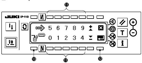
Press 3 in the communication setting screen to display the file No. of media input screen. Input the file No. of media with 1. The file No. which has been inputted is displayed in 2. The No. is determined with 12 after inputting the file No.
